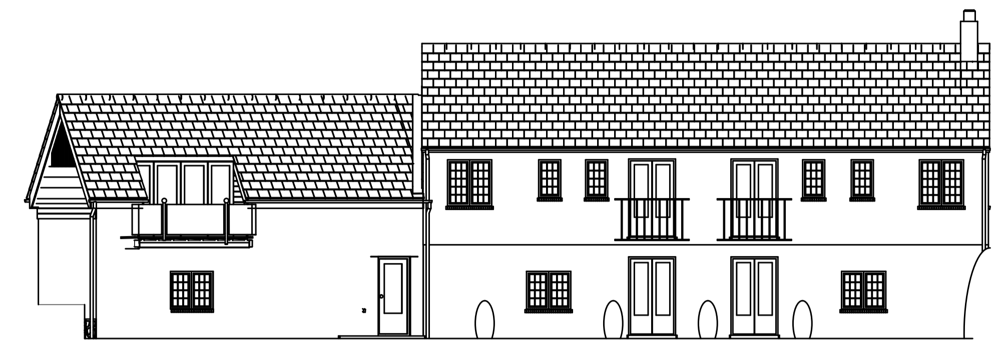
Proposed - Back Elevation Existing Gas Bottle Shelter To Be Removed & Cooker Changed To All Electric
