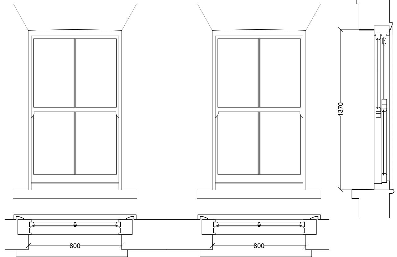
02 FIRST FLOOR FRONT WINDOWS WF-01 & WF-02 AS EXISTING
