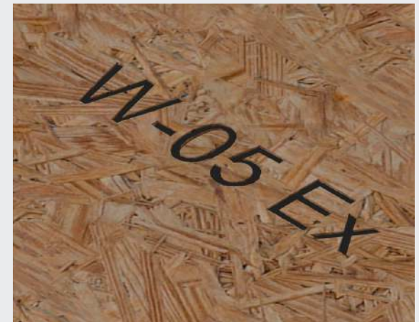
Unique component references guide the off-site assembly and on-site installation process.
