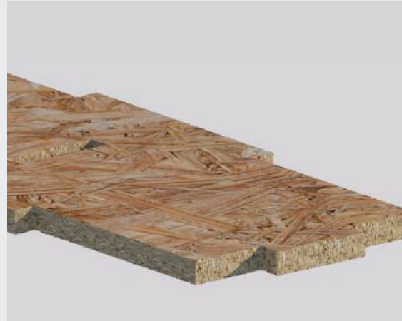
Castelated connections and internal ribs create a structural cassette, removing the need for any internal softwood supports.
