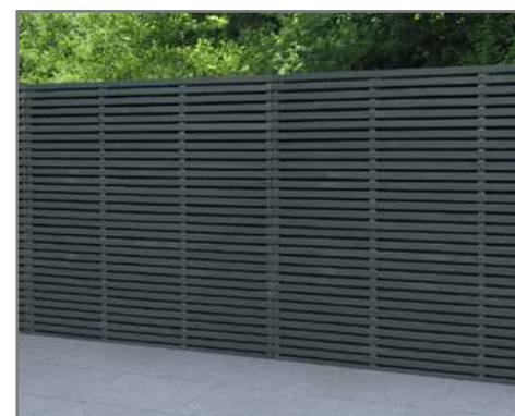
1.8m Forest 'Contemporary' Fence between rear plot boundaries with matching gates. Step as necessary and use planed gravel board and posts stained to match.
