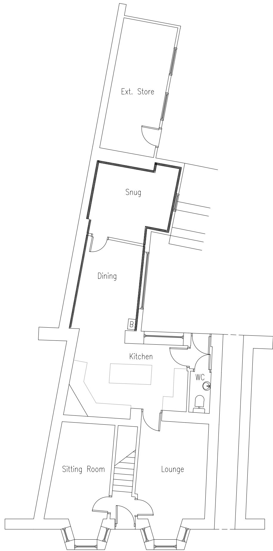
Proposed Ground Floor Plan
