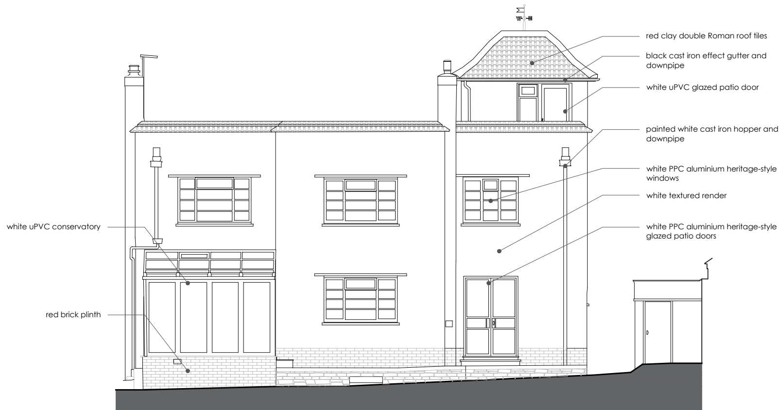
EXISTING SOUTH ELEVATION
