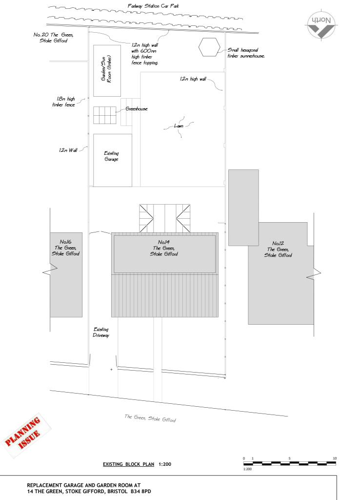
DRAWING No. BR 02 - EXISTING BLOCK PLAN Rev: A 00/00/202? -
