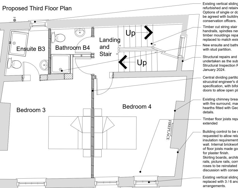
Existing vertical sliding sash window refurbished and retained. Options of single or double glazed to be agreed with building control and
