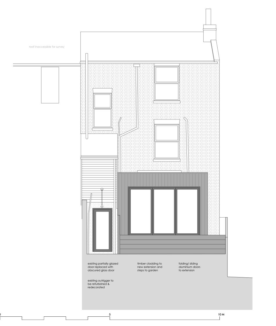
DRAWINGS BASED UPON THIRD PARTY MEASURED SURVEY. ALL DIMENSIONS & SETTING-OUT TO BE VERIFIED ON SITE. ANY DISCREPANCIES TO BE HIGHLIGHTED TO THE CLIENT/ARCHITECT
