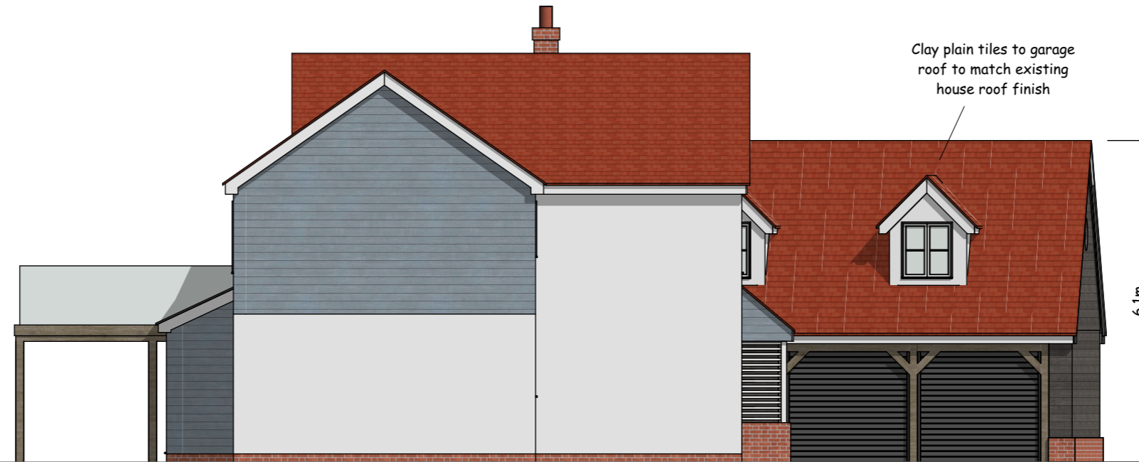
NORTH WEST ELEVATION
