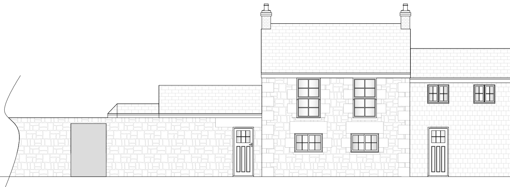
Existing Front Elevation (North)
