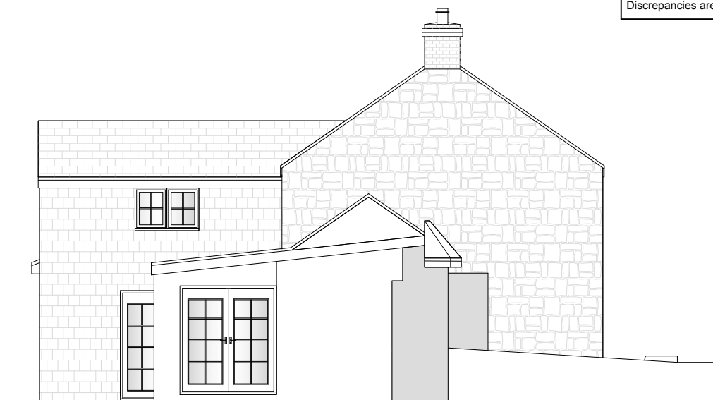
Existing Side Elevation (East)
