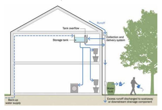
As there is an issue with the storage capability of rainwater harvesting tanks, this method should have a fixed attenuation volume and a controlled outlet to discharge into the proposed infiltration feature. An overflow system will be required for implementation on the Site due to exceedance events (where the pumps fail or there is a blockage within the system / or the number of residents and subsequent water usage is reduced).
