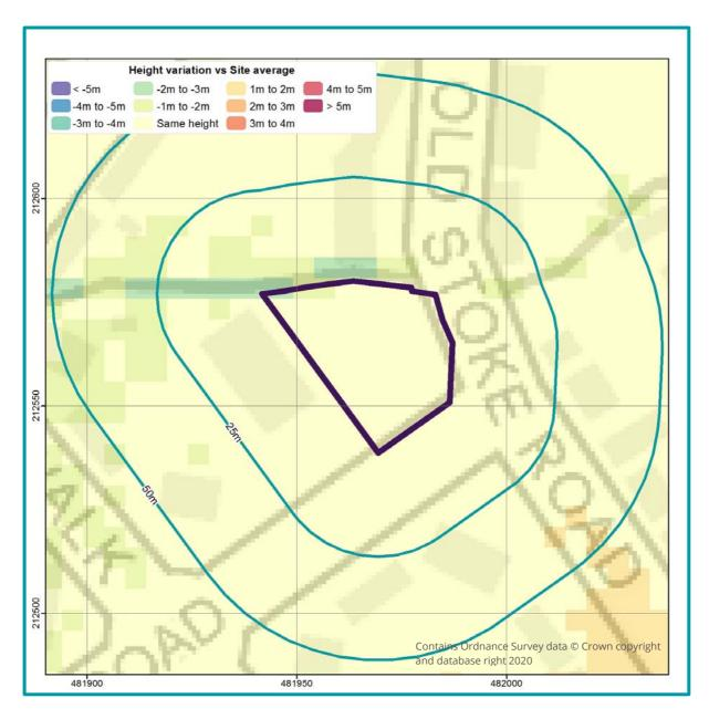
GeoSmart have undertaken an assessment of the topography at the Site and within its vicinity, using LiDAR elevation data from the Environment Agency (EA). The mapping shows a comparison between average ground levels on the Site with ground levels in the surrounding area.
