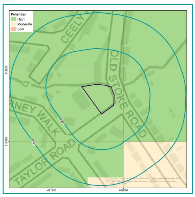
The GeoSmart SuDS Infiltration Suitability (SD50) Map screens the potential for infiltration drainage at the Site and indicates where further assessment is recommended. The map combines information on the thickness and permeability of the underlying material and the depth to the high groundwater table. According to the SD50 map, there is a high potential for infiltration SuDS within the Site.
