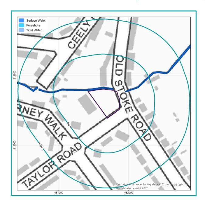
GeoSmart have undertaken an assessment of the location of surface water features within the vicinity of the Site. A surface watercourse is located adjacent to the northern Site boundary. Discharge to surface water is likely to be appropriate.
