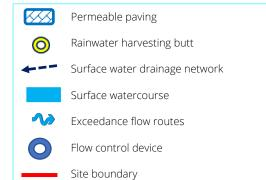
Surface water runoff from the proposed development roof and car park/paving should be conveyed into the proposed permeable paving where it can be attenuated prior to discharging to the nearby watercourse.
