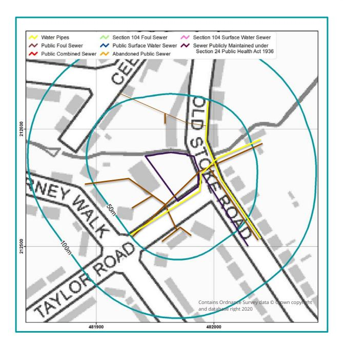
GeoSmart have undertaken an assessment of the location of sewer features within the vicinity of the Site. The Site is situated further than 100m from a public surface water or combined sewer. Discharge to sewer is unlikely to be appropriate.
