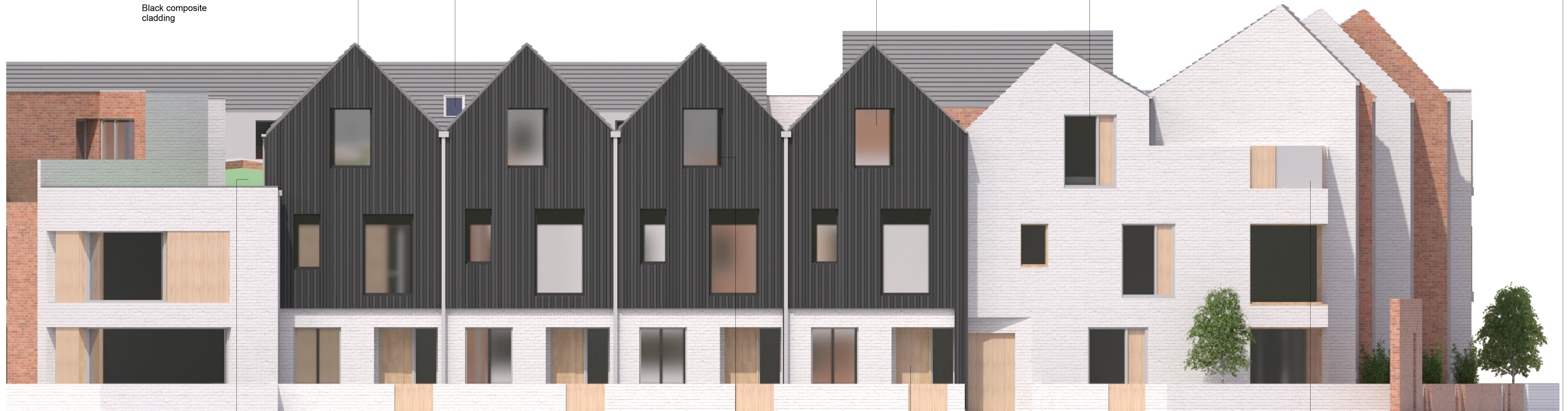
Window reveal consists of white painted brickwork.
