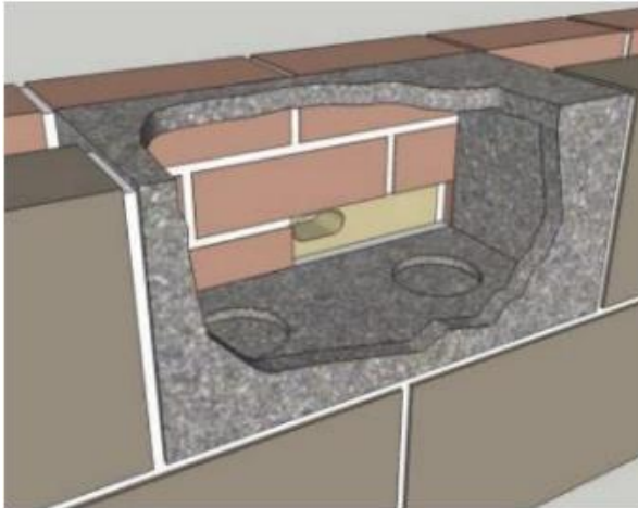
Figure 6. A schematic of how the Cambridge full face Swift brick leads into a cavity created by the prior installation of the Swift maxi nesting box.
