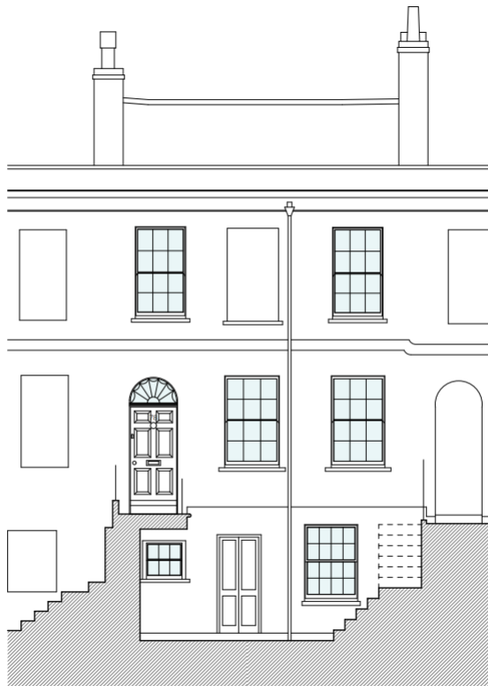
Figure 3 Front Elevation and steps section
