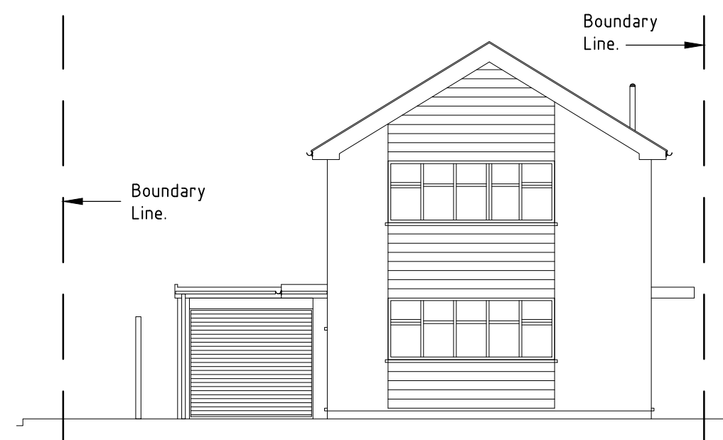
EXISTING FRONT ELEVATION ( 1: 100 )
