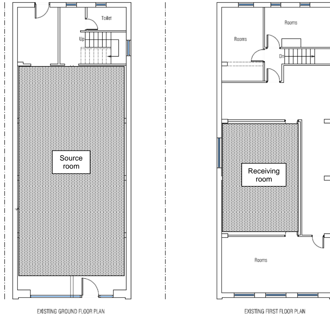
Figure 2. Existing ground and first floor layouts
