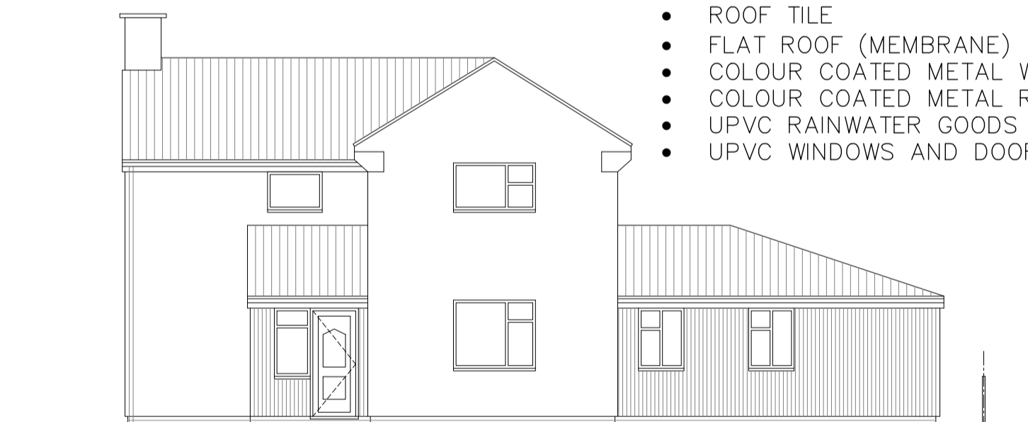
09 PROPOSED FRONT ELEVATION 1:50 @ A1
