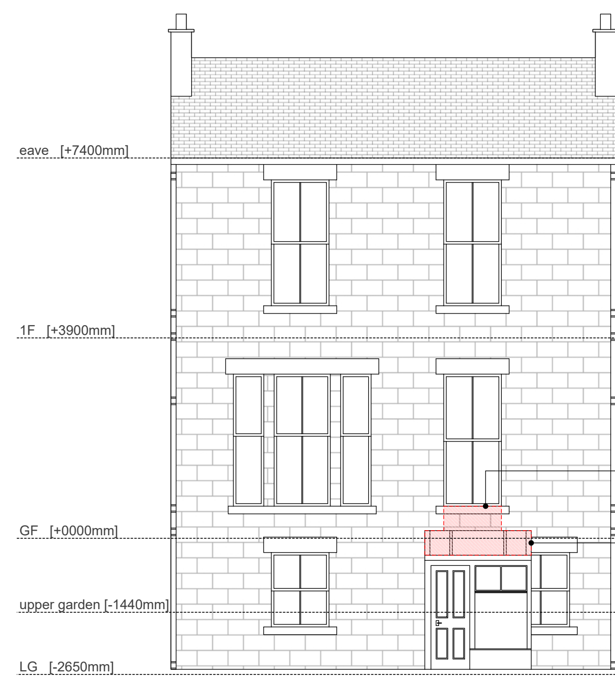
04 Existing North Elevation 0100 1:75
