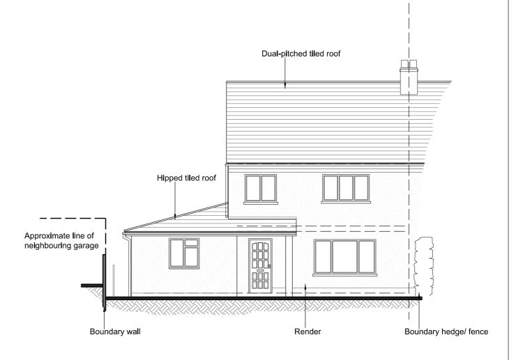
EAST ELEVATION WEST ELEVATION
