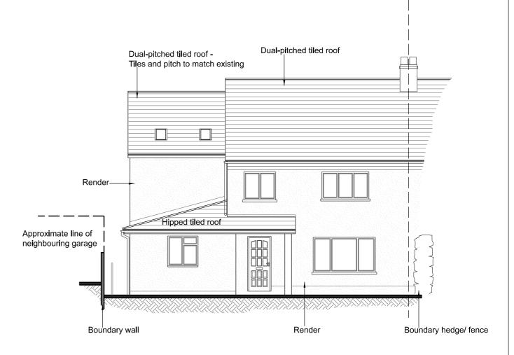
EAST ELEVATION WEST ELEVATION
