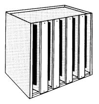
are manufactured from galvanised sheet steel and have slides for the insertion and removal of individual carbon panels. The panels have an aluminium channel frame surround to prevent damage to the panels. when being inserted, and to provide a base for sealing gaskets.
