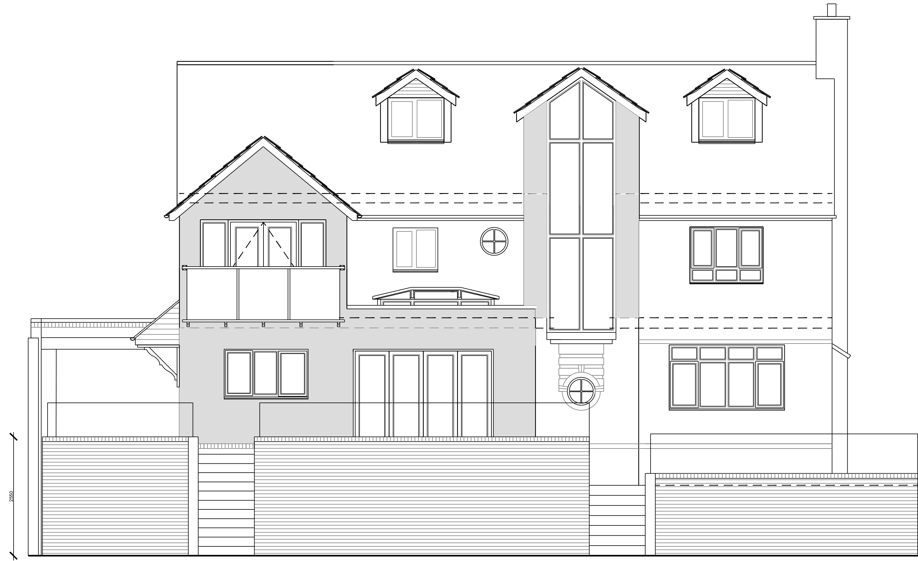
Rear Elevation (indicating retaining walls)
