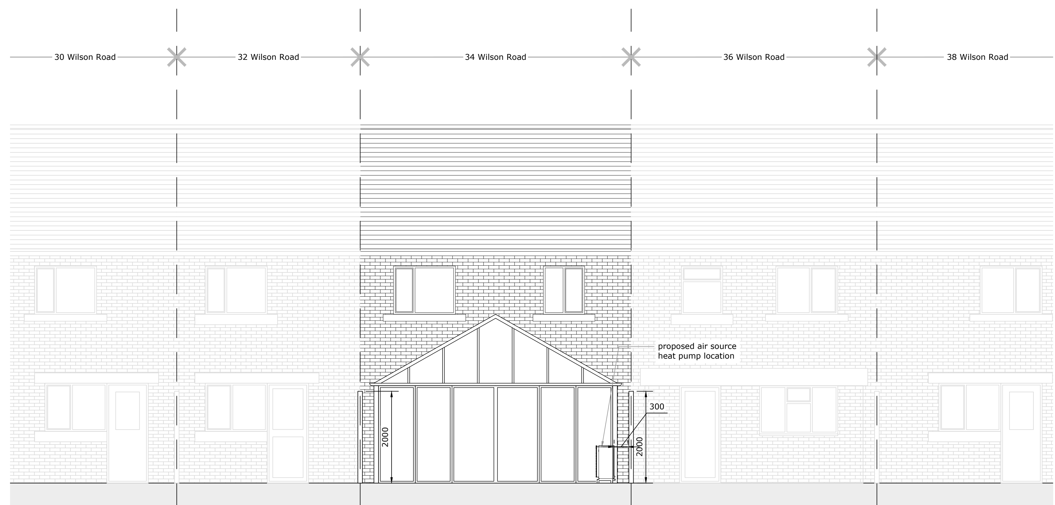
rear elevation (south facing) as proposed 1:50
