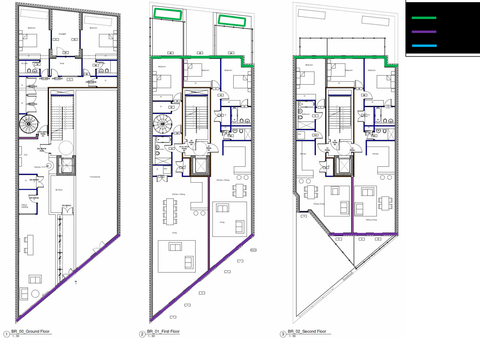
FIGURE A1: SITE WIDE GLAZING ZONING PLAN – GROUND FLOOR TO SECOND FLOOR
