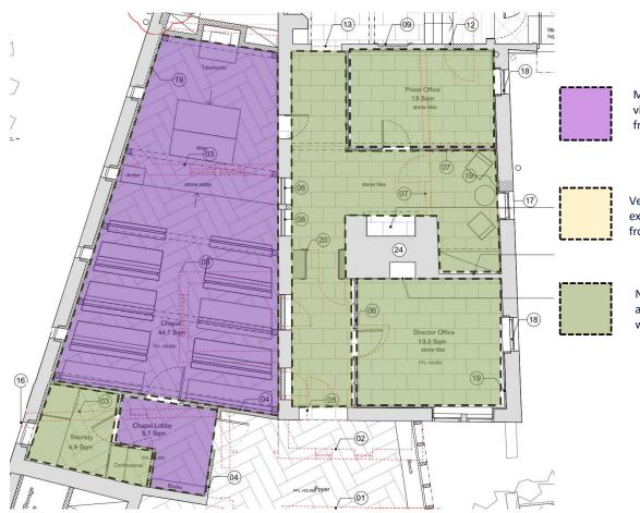
Mechanical Supply Ventilation via MVHR + natural ventilation from openable windows
