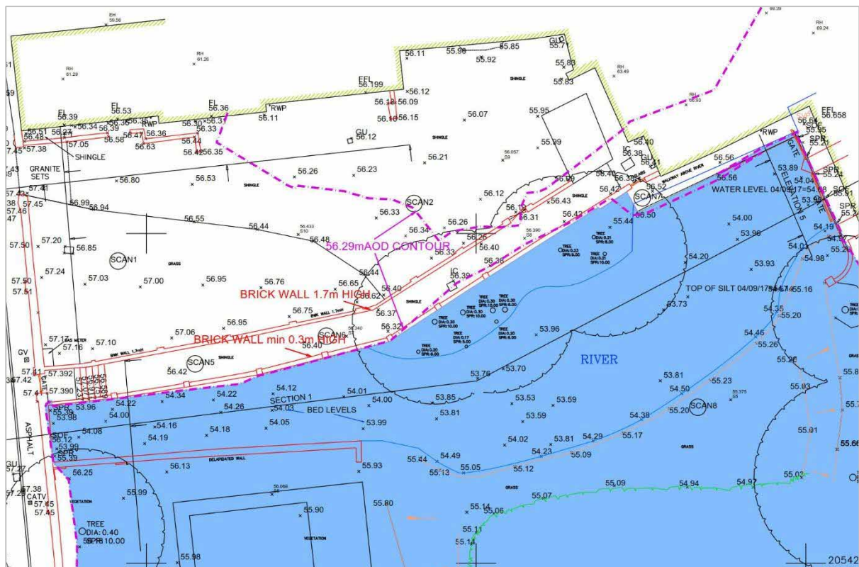
Figure 5: Topographic Survey and Flood Levels
