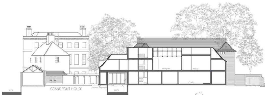
SECTION 10/00A LONG SECTION ACROSS NEW BUILDING AND LINK CORRIDOR
