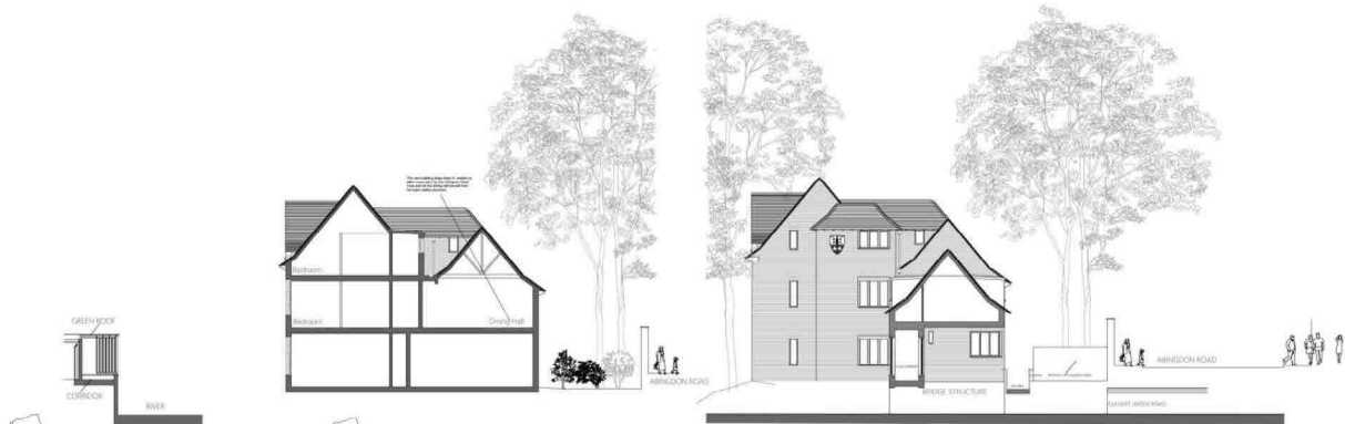
SECTION 10/00A LONG SECTION ACROSS NEW BUILDING AND LINK CORRIDOR
