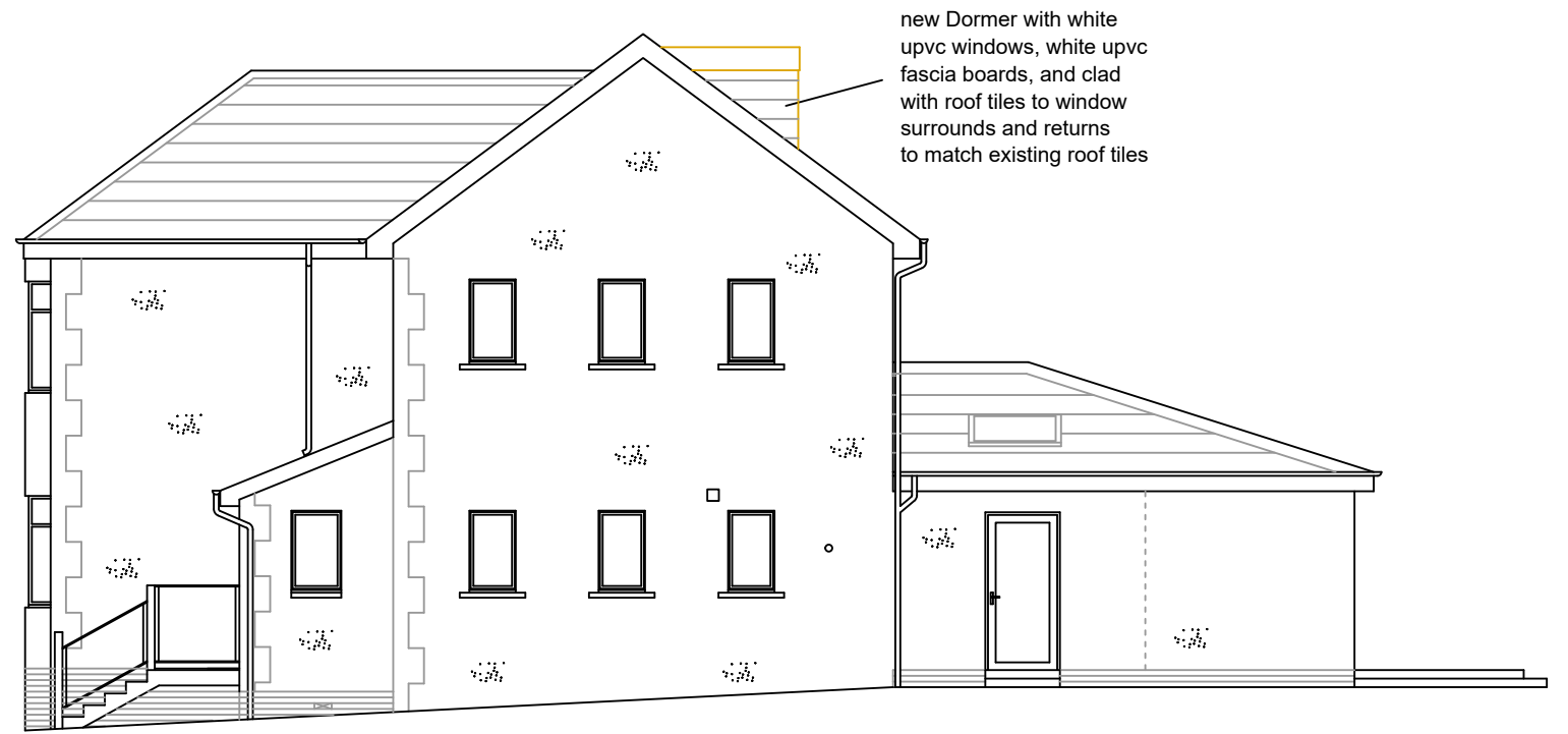
SOUTH ELEVATION AS PROPOSED
