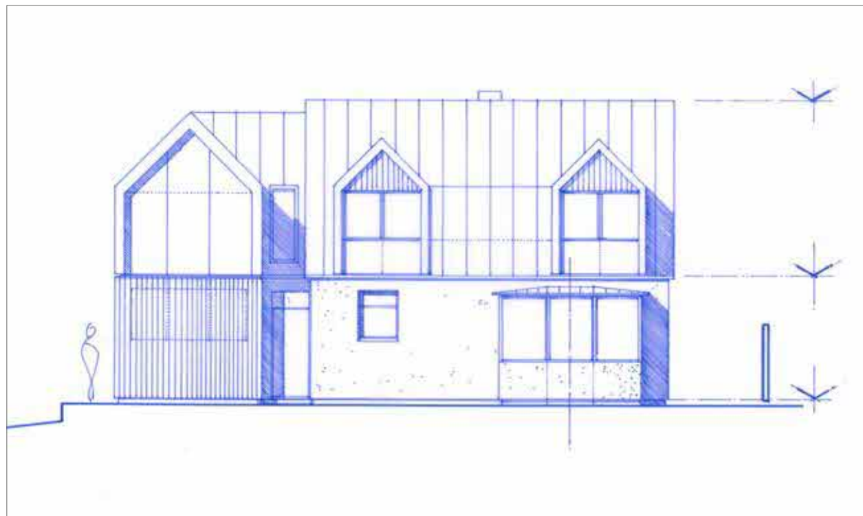
Proposed Elevation to Bourne Lane - New Dormers in Existing Roof and Outshot Extension
