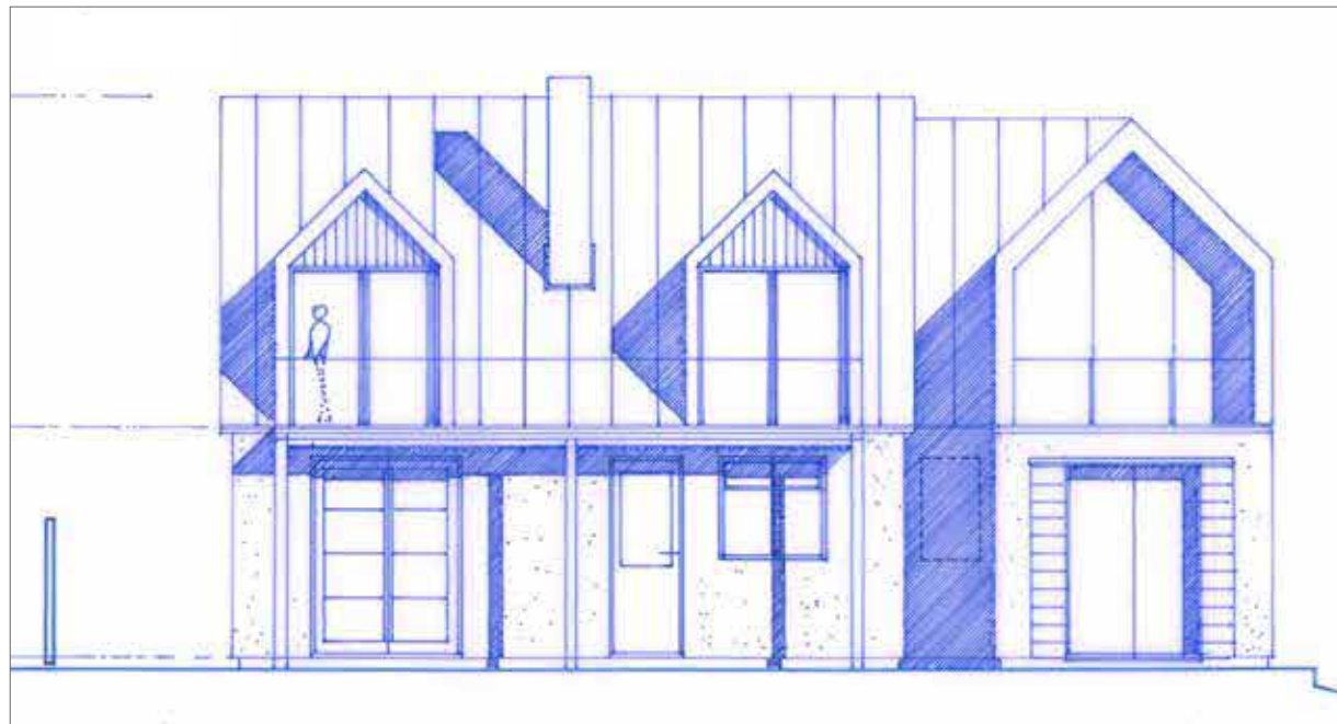
Proposed Elevation to Rear Garden - New Dormers in Existing Roof and Outshot Extension
