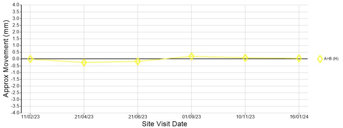
C2 - INT - Cracking to chiney breast THS
