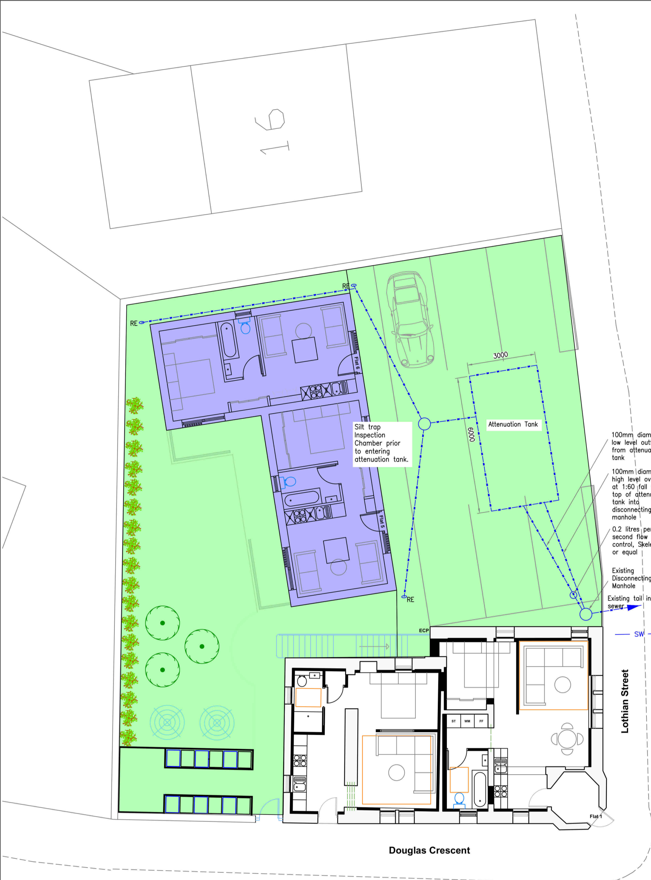
SURFACE WATER DRAINAGE PLAN (Scale 1:100)
