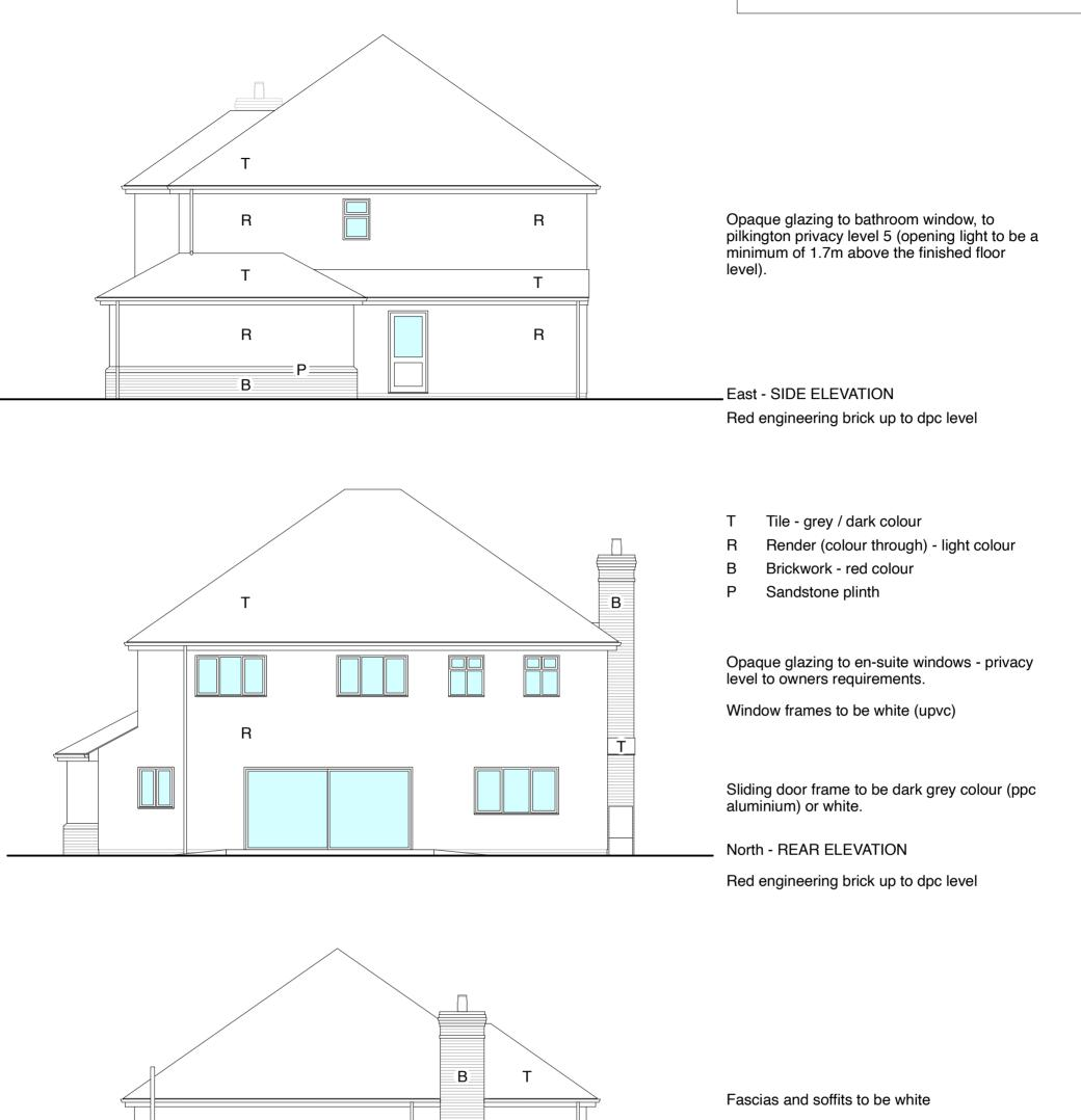
Rainwater gutters, pipes and S+VP to be black / dark colour
