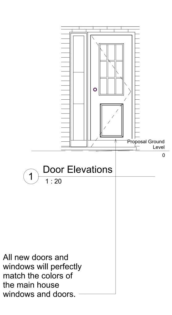
New and replacement doors to achieve a U-Value of 1.4W/m<sup>2</sup>K. Glazed areas to be double glazed with 16-20mm argon gap and soft low-E glass. Glass to be
