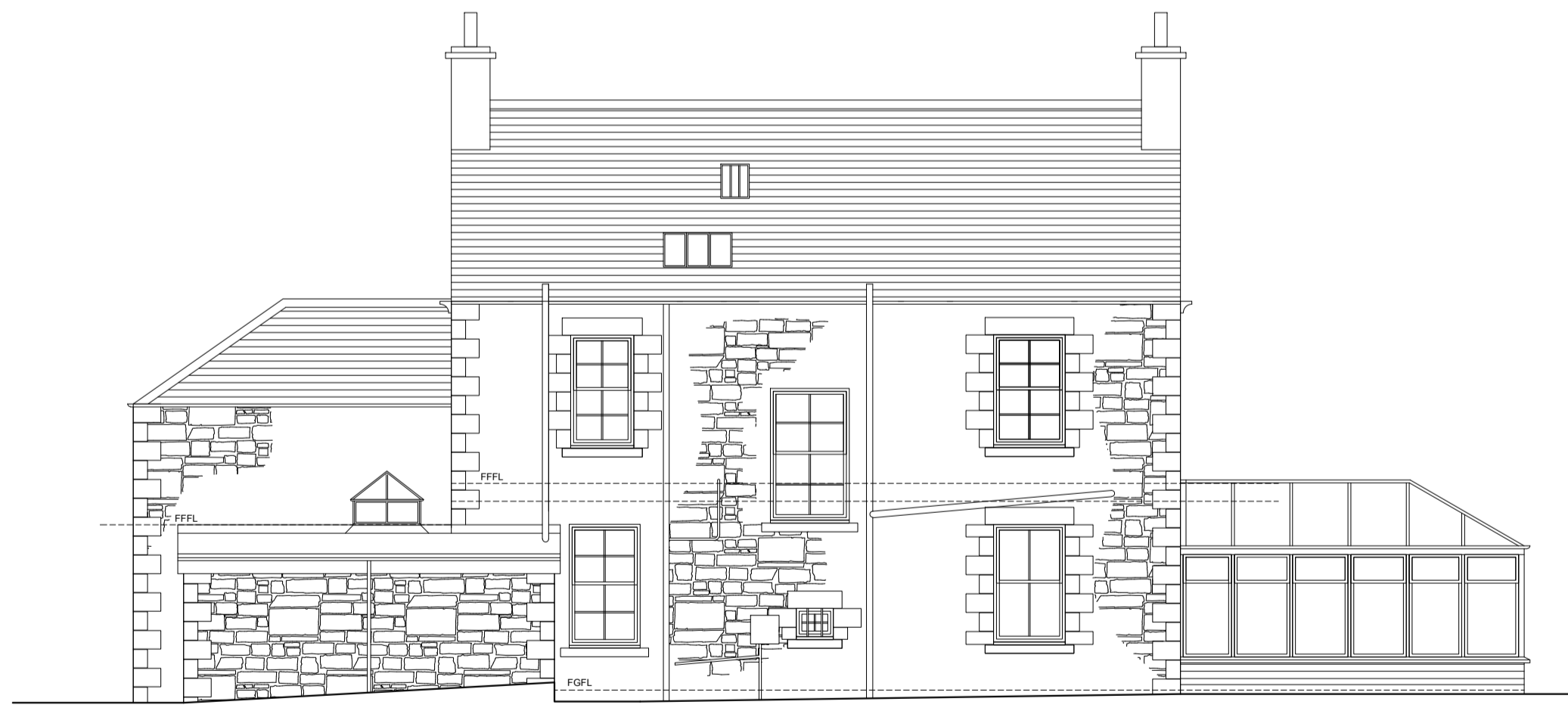
NORTH ELEVATION (REAR) AS EXISTING SCALE 1:100
