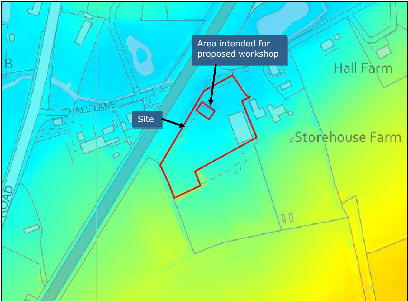
Figure 2: Filtered LIDAR survey data at 1m resolution where higher ground is denoted by red and orange colours and lower ground is denoted by blue colours
