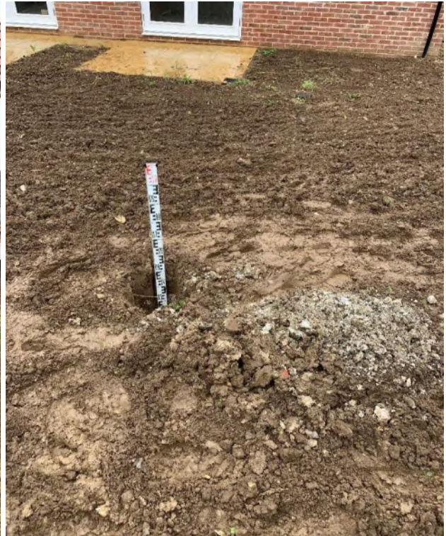
Photographs 1-2 , taken on the 01 st September 2023 showing examples of hand dug trial pits and the nature of the subsoil and topsoil within the soft landscaping of plot 88 (back garden).
