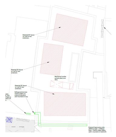
The approximate area of panels that could be installed would be **50m2**. This provides around 10kWp.
