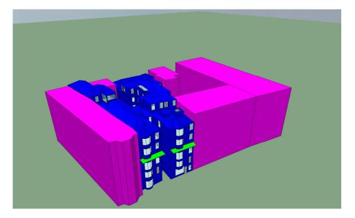
The thermal model has been set up using the standard SBEM profiles for a student accommodation building to provide the energy demand for the regulatory items – heating/cooling, ventilation, lighting, hot water.
