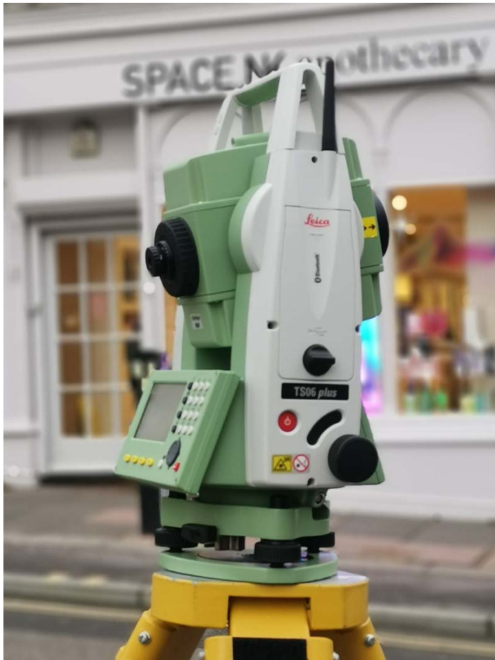
Fig 5: Total Station TS06+ used for data collection
