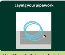
Using blue polyethylene (mdpe/pe) or barrier pipe - lay a continuous unjointed length of pipework to the boundary with the public highway ensuring there is a sufficient length of pipe to allow for an unjointed connection to the host main unless instructed otherwise.
