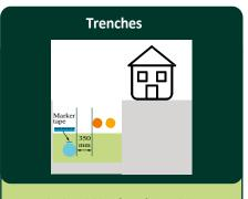
Trench should be free from debris and wide enough (350mm) to accommodate the pipework it is hosting together with any other utility services sharing the same trench. Please see G4.15 R4.15 in Schedule 2 of the Water Regulations for more information.
