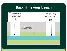
The trench should be lined and filled with fine granular backfill or selected soft earth free from rubble and waste. The trench should remain open until it has been inspected.
