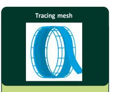
The mesh must be visible on site at inspection, and is to be installed approximately 350mm below finished ground level.
