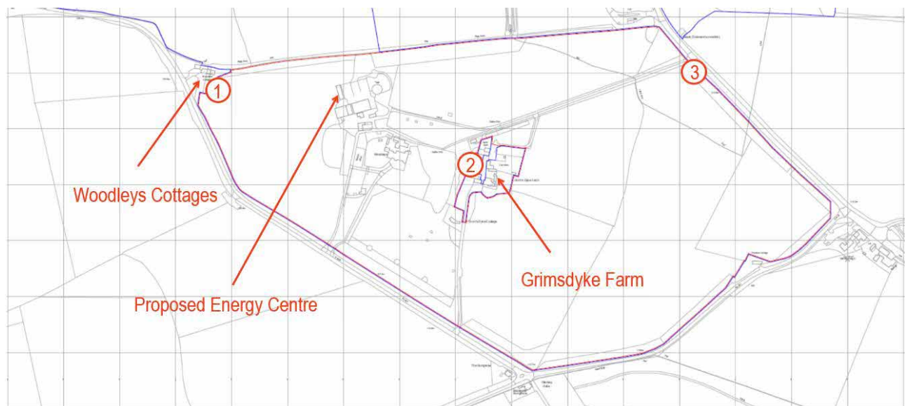
Figure 2. Environmental Noise Monitoring Positions and Nearest Adjacent Residential Receptors
