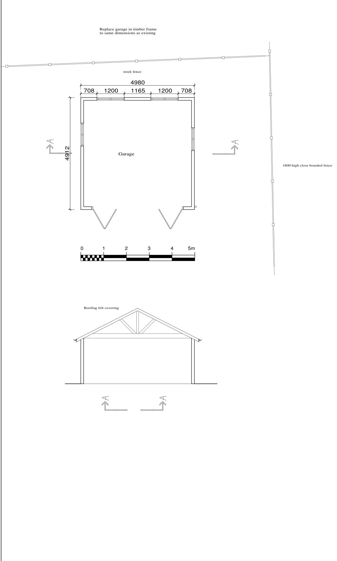
Roof in felt shingles to match existing. Walls in timber Shiplap to match existing. Windows and doors in timber.
