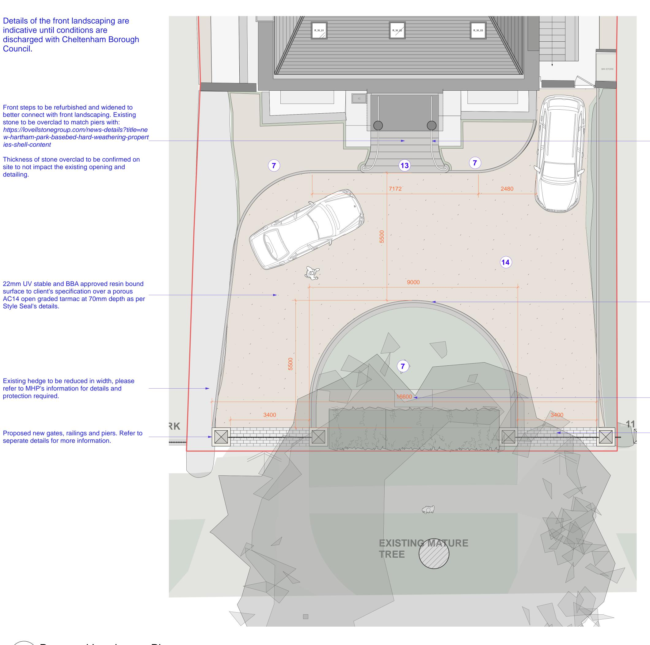
Black painted iron railings and balustrade to match the proposed gates (L(9)11 & 12). Detailed design to be confirmed by specialist manufacturer and confirmed with client prior to manufacturing.
