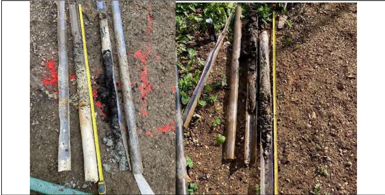
Core runs of BH601 (left) and BH603 (right)
