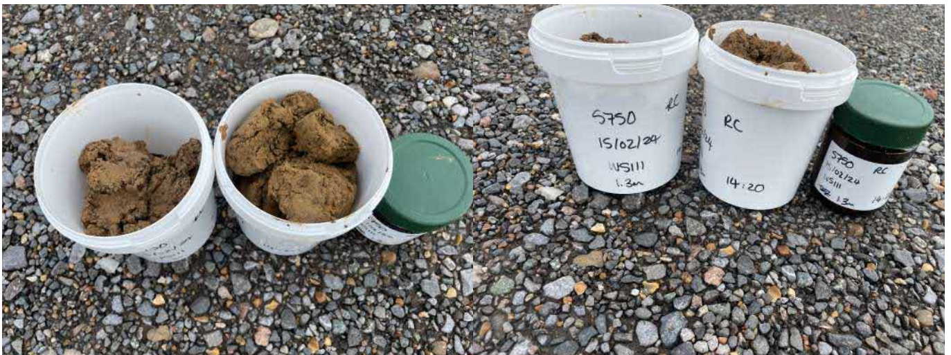
Photo 6—Examples of disturbed soil samples taken at WS111 for chemical analysis
