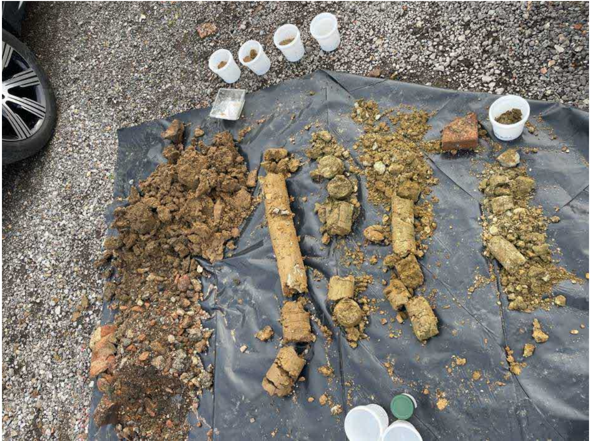
Photo 5—Example of hand dug safety starter pit arisings and cores up to 5m bgl
