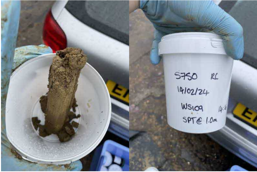
Photo 7—Example of Standard Penetrations Test (SPT) arising from WS109
