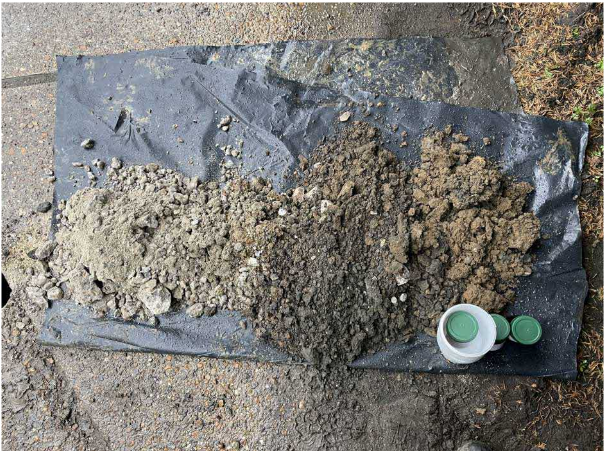
Photo 4—Example of the arisings from a hand dug safety starter pit
