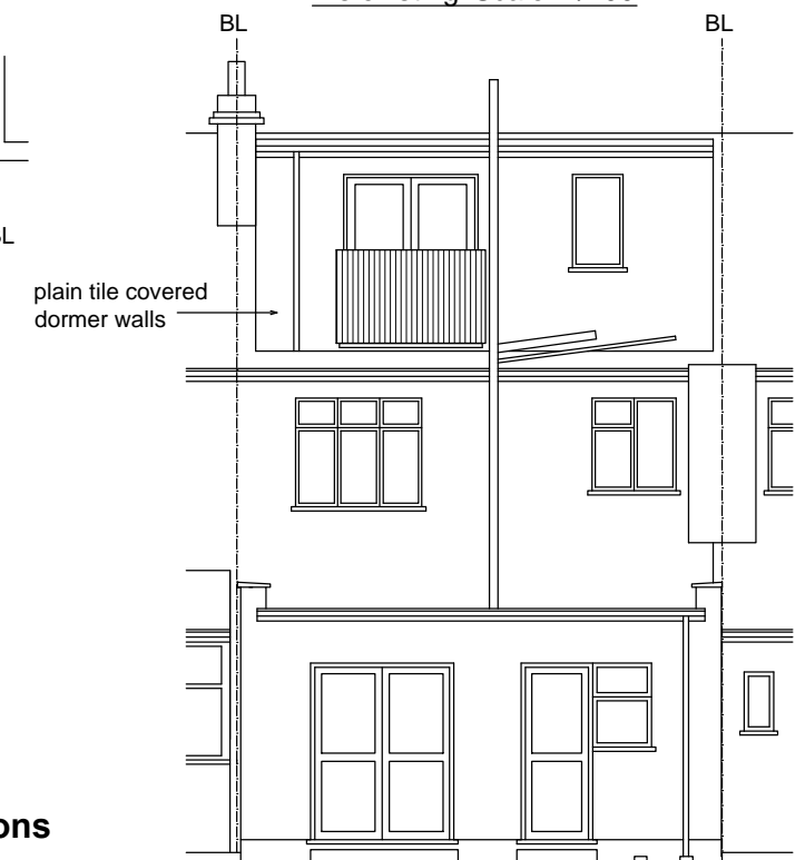
Rear Elevation 'As existing' Scale: 1/100
