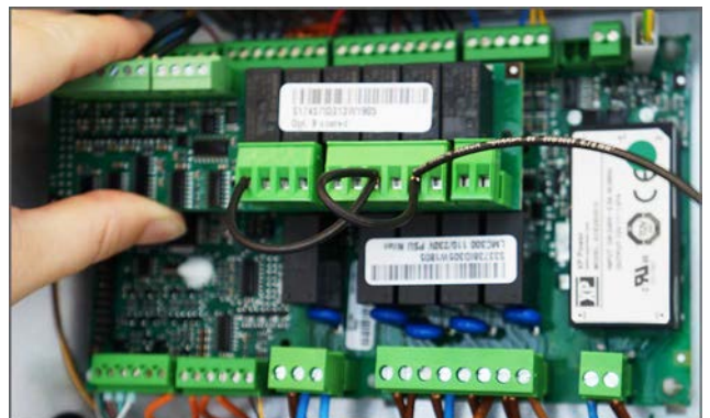
4. Mount the expansion PCB on the CTS602 Light circuit board.
