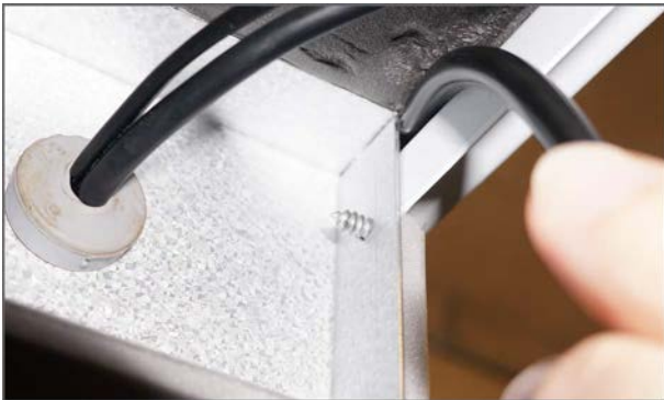
3. Pierce a hole into the foam over the crossbar, (where the heat exchanger is positioned) to gain access to the recess in the top cover.
