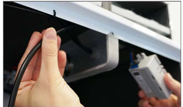
4. Run the wire from the CO 2 sensor through this recess.
