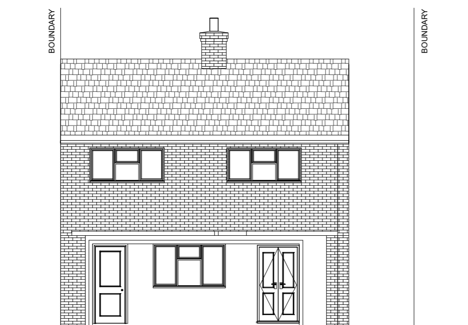
EXISTING REAR ELEVATION
