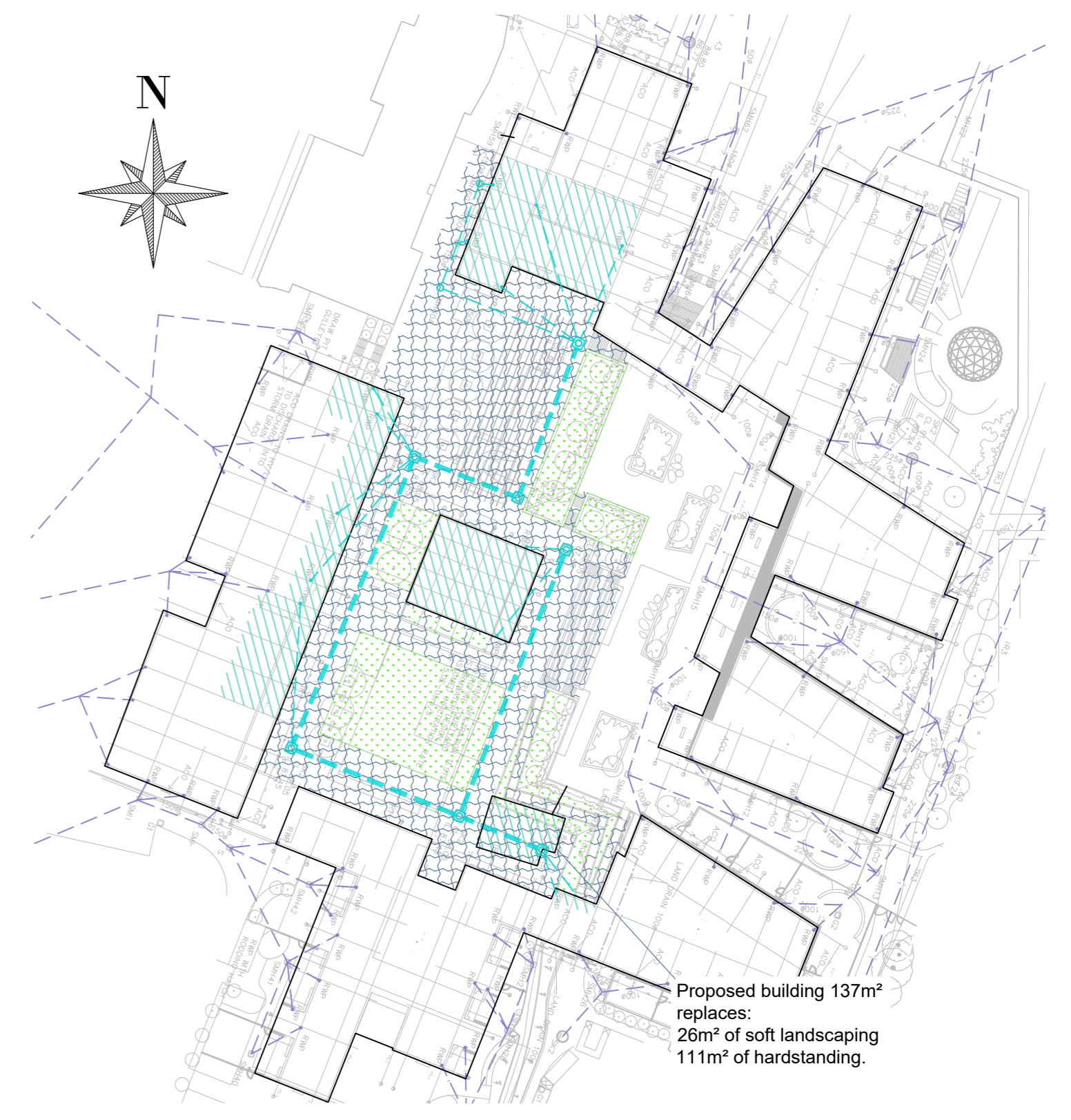
Contributing Areas for the drainage system to which the proposed building will connect
