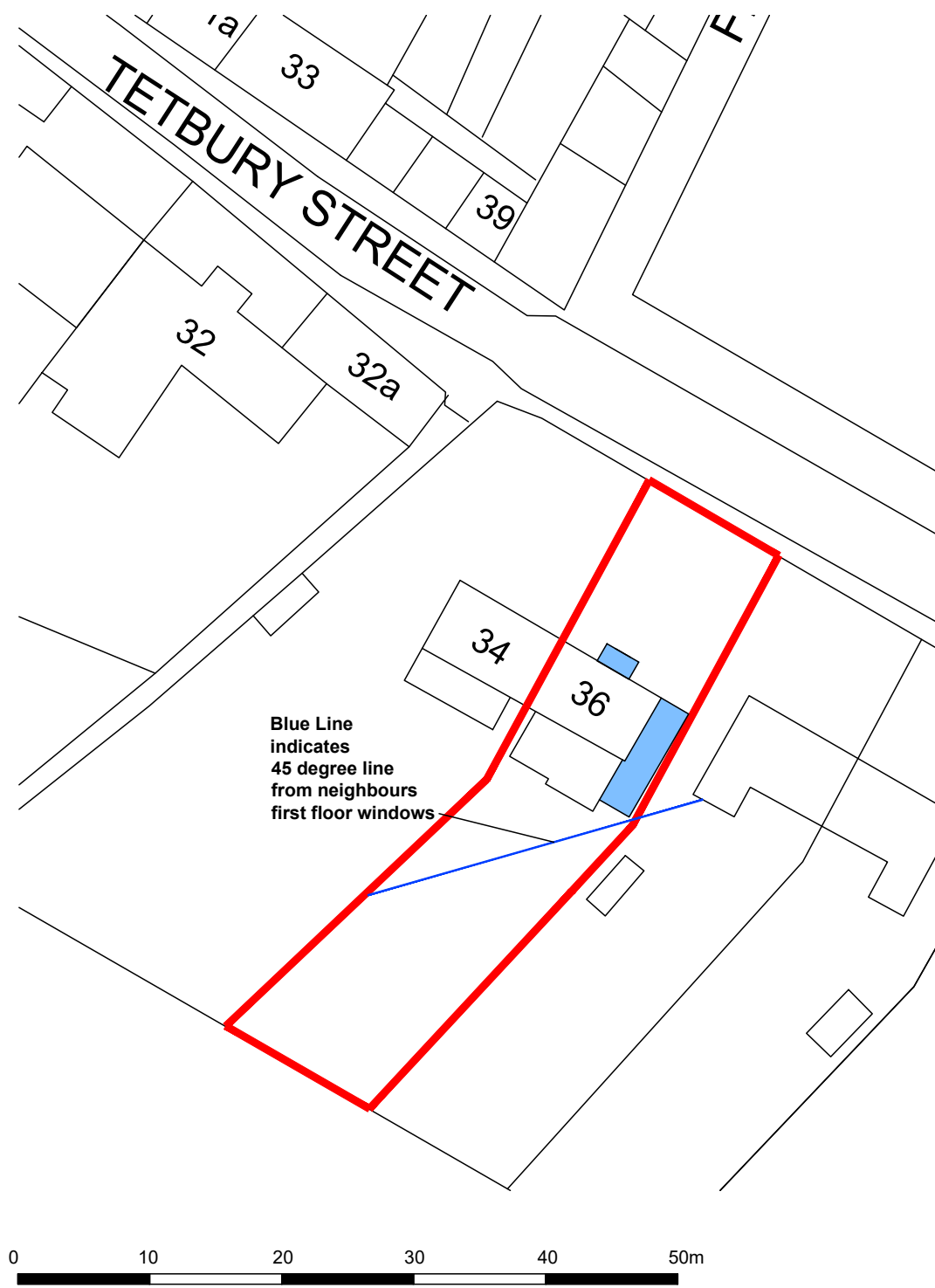
PROPOSED BLOCK PLAN - 1:500
